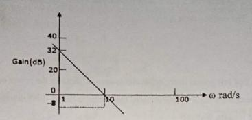
The gain (20 log G(s)) is 32dB and -8dB at 1 rad/s and 10 rad/s respectively.
